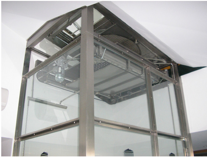
Fig. 6. Rain room and vertical rain generator.
